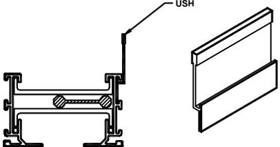
Suspends one side of the FlowBar assembly from the ceiling structure.
